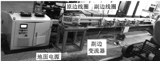
图 8 实验样机图 Fig.8 Prototype of IPT system
