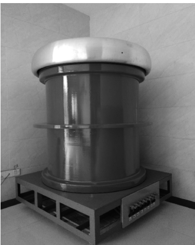
图 16 200 kV,100 kV·A 磁控谐振变压器样机 Fig.16 Prototype of 200 kV,100 kV·A magnetically controlled resonant transformer
