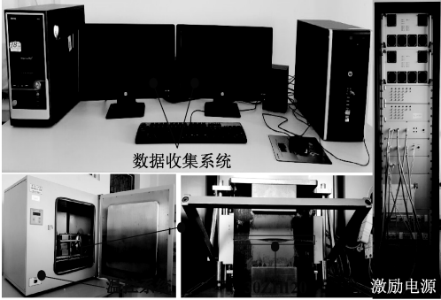
图 1 电工硅钢片磁特性测试设备 Fig.1 Test equipment for magnetic characteristic of electrical silicon steel
