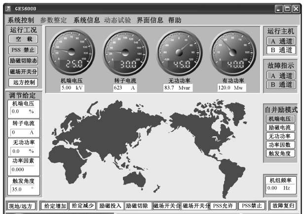
图 6 商用人机界面上显示的励磁控制器连接情况 Fig.6 Operation status of proposed excitation controllers monitored by commercial HMI
