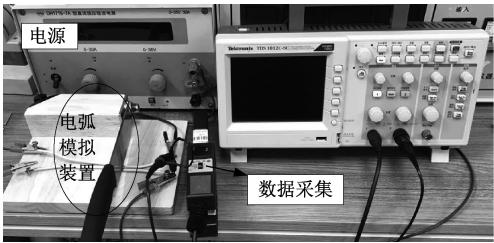
图6 并联故障电弧装置 Fig.6 Parallel fault arc generator
